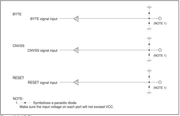
Figure19.6 I/O Pins
